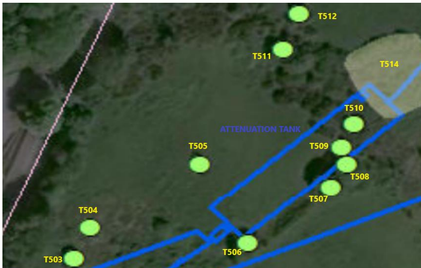
FIG 5 – Trees in conflict with attenuation tank
